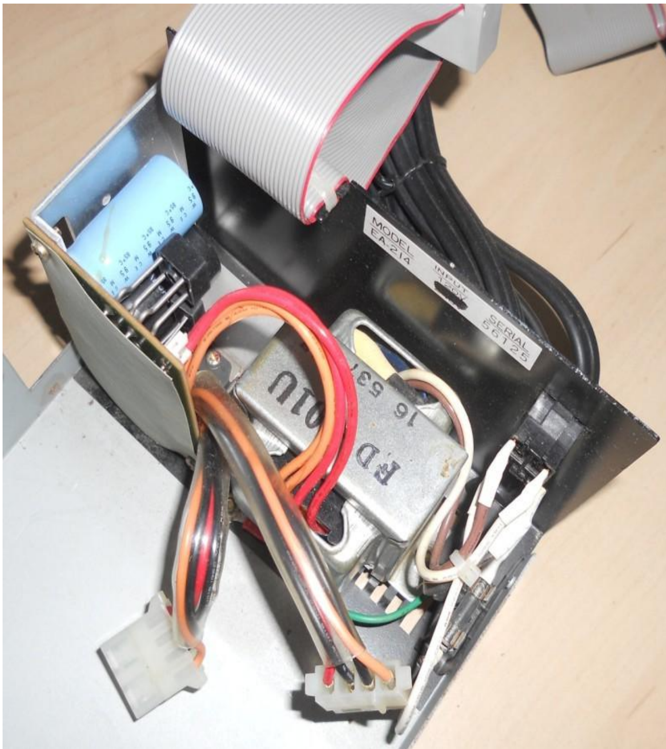
Picture: shows transformer and is joined to regulator via red and orange wires
