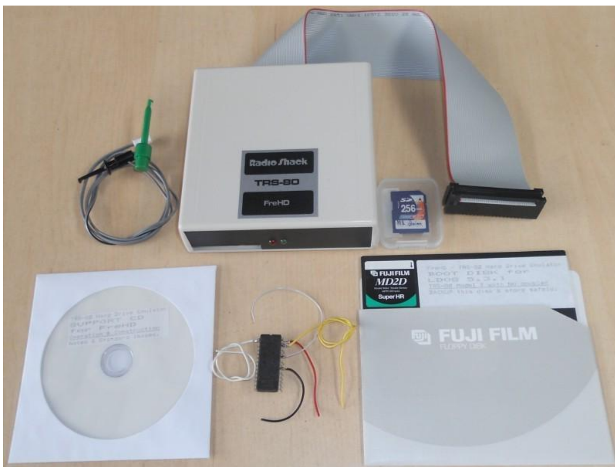
Picture: FreHD/M1HD adapter Combo box for the expanded Model I system
