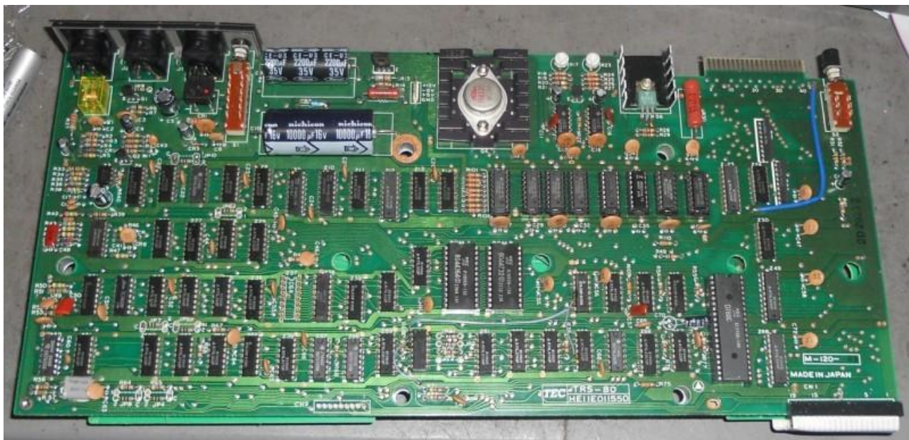
Picture: J1 motherboard by TEC (shows RAM sockets, installed by previous owner - standard J1 has soldered in RAM chips)
