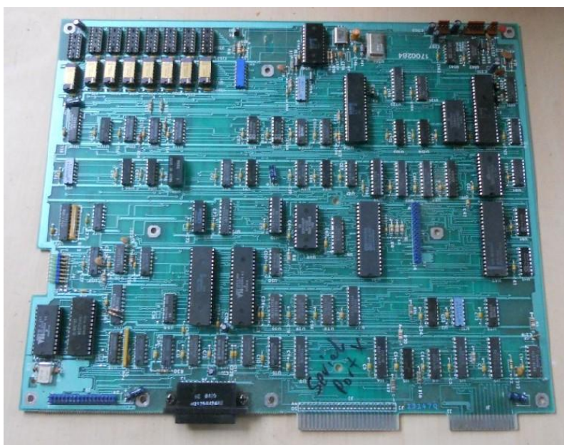
Picture: 4P Gate-Array motherboard, 4P Non-Gate Array motherboard is similar.
