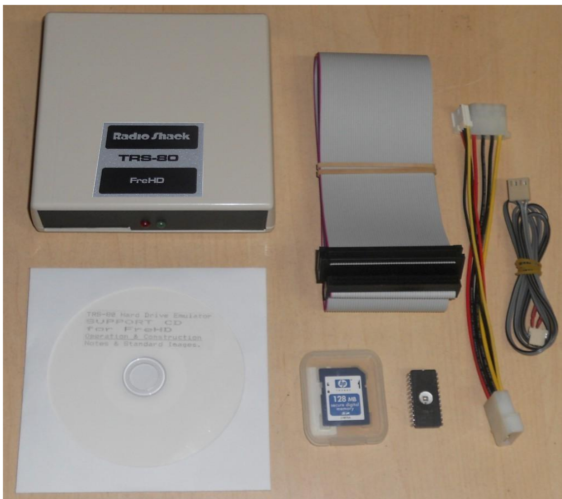
Picture: FreHD kit for the Model III, 4, 4P and 4D includes Eprom and power cables
