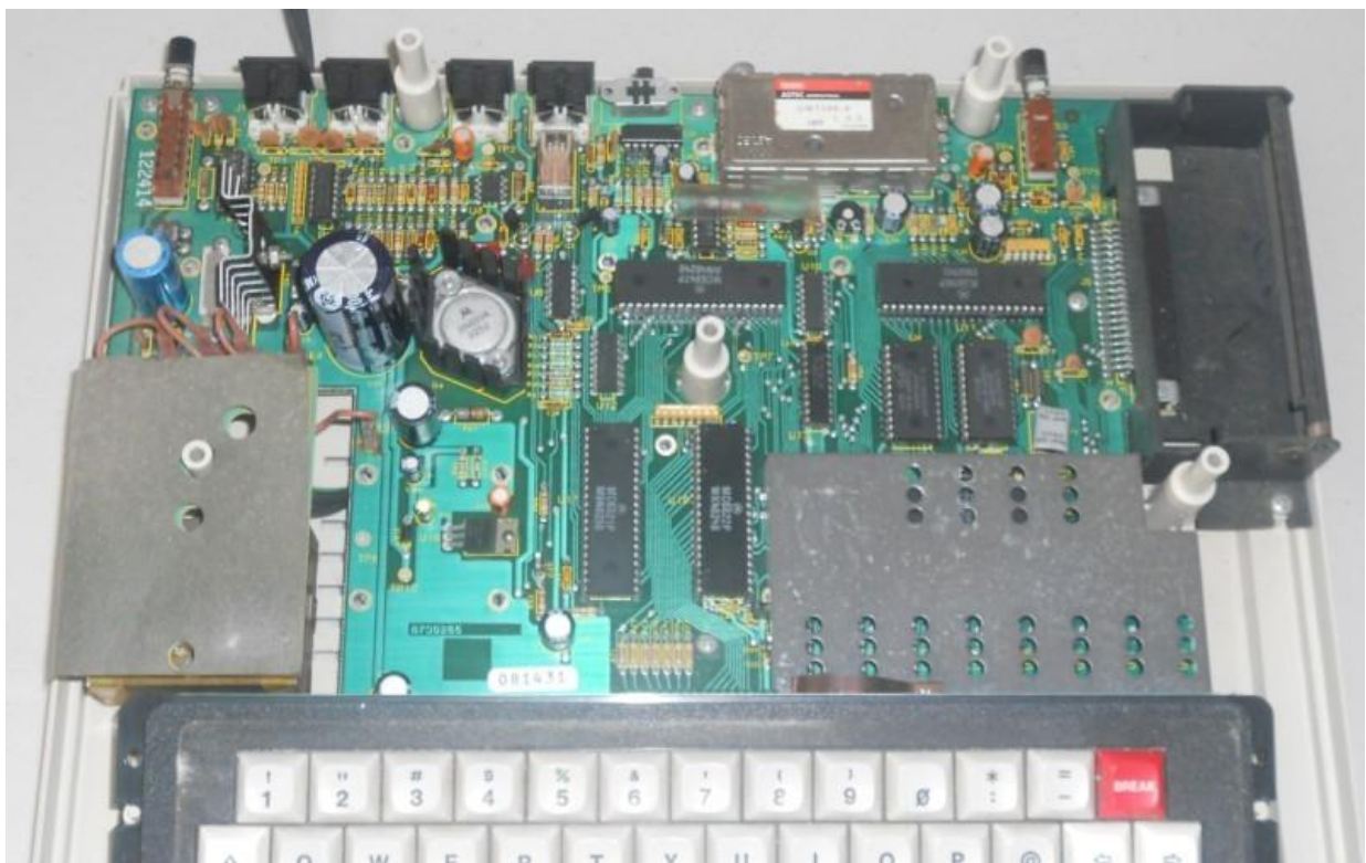
Picture: inside the US 64K Color Computer features the "285" aka "F" motherboard
