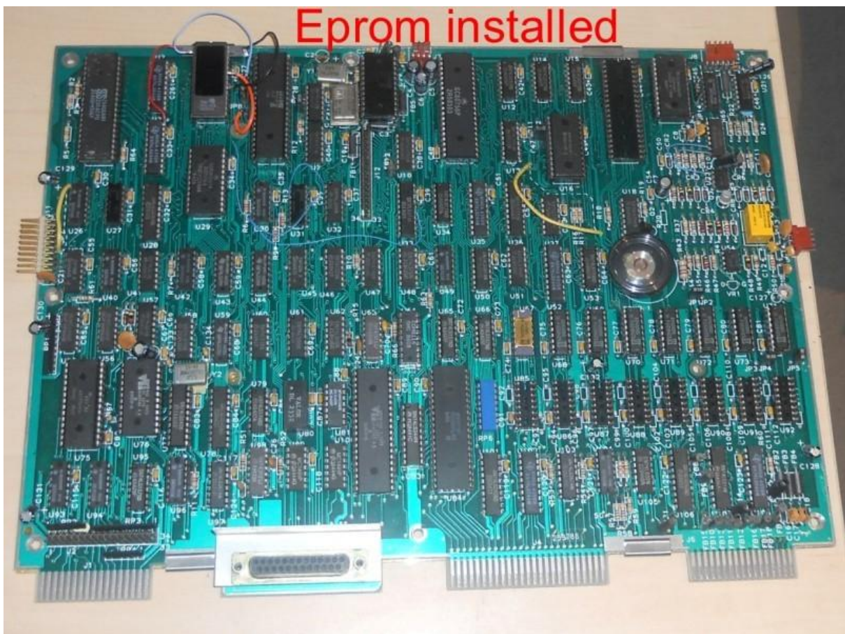
Picture: completed modification and motherboard ready to re-install in the computer.
