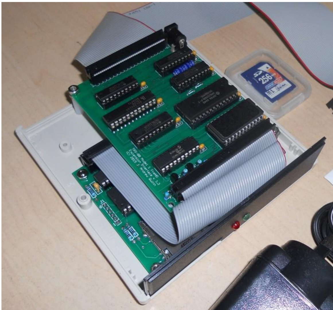
Picture: how the FreHD and Quininterface are packaged inside the heavy-duty plastic box
