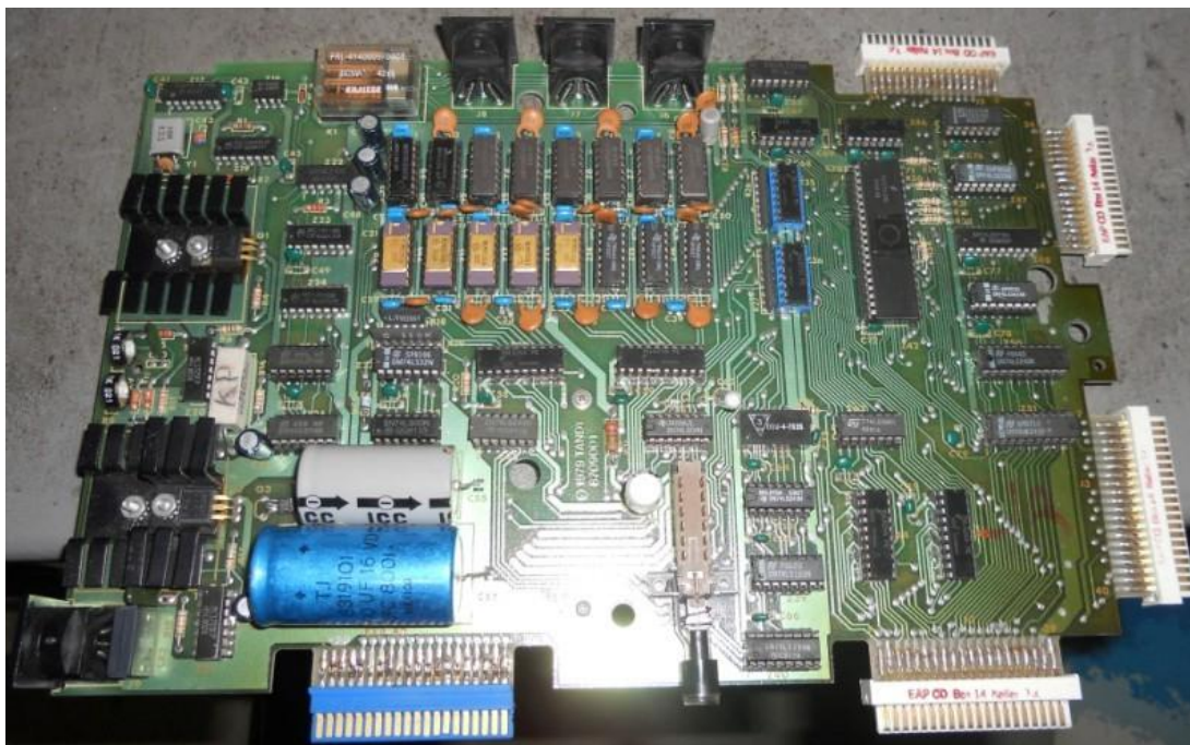
Picture: Re-designed EI shows parts layout. This one has Goldplug-80s (good) and mismatched RAM (bad)
